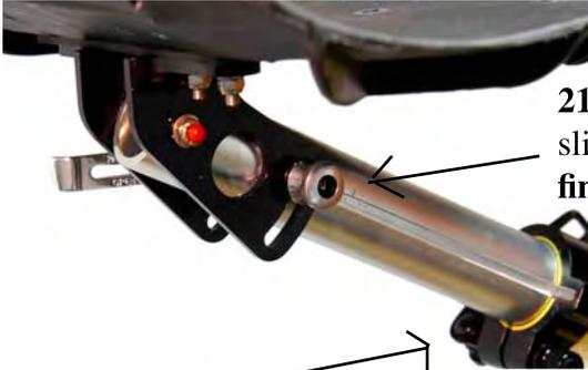
**21.** Adjust seating seat tilt by releasing Q.R. clamp and sliding to the angle that suits you. **Note: See riding tips for fine tuning seat adjustment.**
