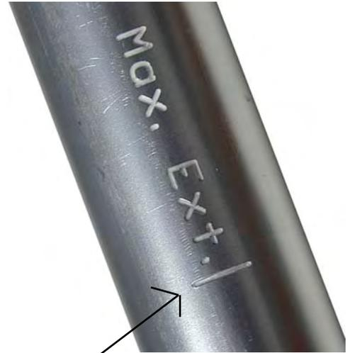
**Warning: Do not raise seat post height past max extension mark located on the seat post.**
