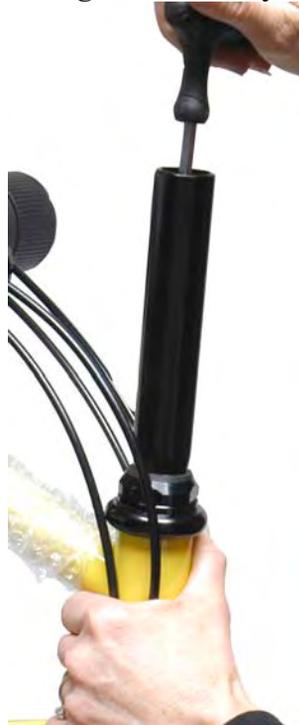
**13.** Loosen Clamps on Handlebar with 5mm allen wrench prior to putting riser on stem.
