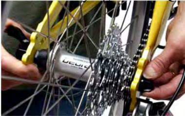
Turn RH shifter to highest gear to position chain on smallest sprocket.
