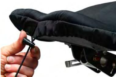
**22.** Slip on seat cover pinching the barrel lock and pulling cords to tighten around the seat. Snip off extra cord or tuck into seat cushion.
