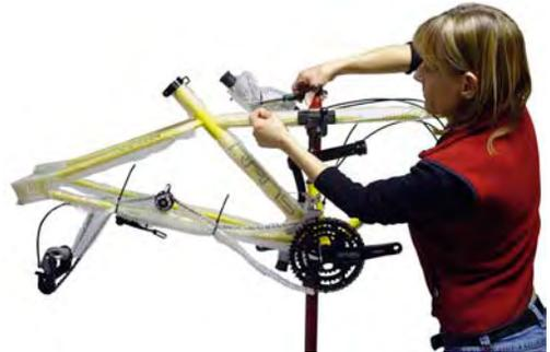
**12.** Insert the stem riser into the fork. You might have to take the stem and loosen it with a 6mm allen wrench prior to putting it in the fork. Hold the stem in place while securley tightening the stem bolt. Hold one hand on the stem and the other on the fork. You should not feel any play between the fork and stem. (Make sure the stem is inserted fully into fork.)
