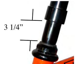
**Do not over extend height of bar. Gap between the riser clamp and headset lock nut should be no more than 3 1/4\"/>**
