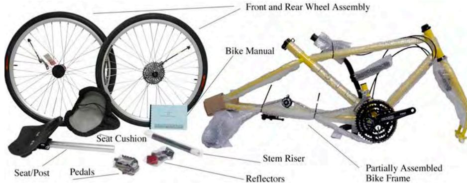
1. Remove the bike and all parts from the carton, then lay out unassembled parts.
