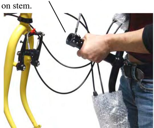
**14.** Take the handlebars and riser, slide onto the stem. Tighten square to fork with fork forward.
