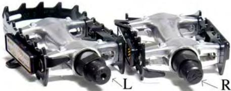
**Note: Start each pedal by hand to avoid stripping the threads.**
